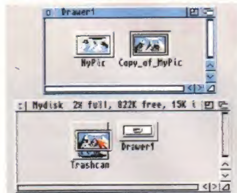
One way to get rid of a file is simply to sling it into the Trashcan, then empty the trash.
